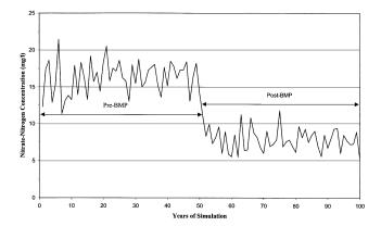
Figure 9–Comparison of pre-BMP and post-BMP annual average nitrate-nitrogen concentrations in leachate at Site D.
