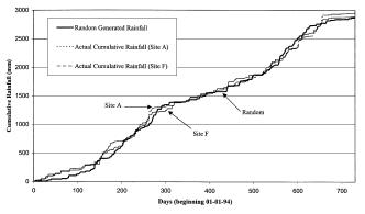
Figure 4–Comparison of randomly generated rainfall versus measured rainfall at Sites A and F.
