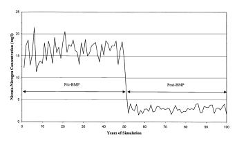
Figure 5–Comparison of pre-BMP and post-BMP annual average nitrate-nitrogen concentrations in leachate at Site B.
