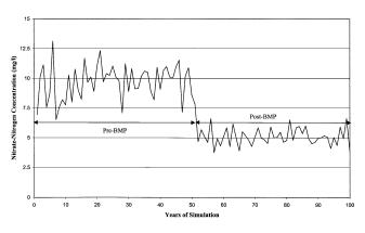
Figure 7–Comparison of pre-BMP and post-BMP annual average nitrate-nitrogen concentrations in leachate at Site C.
