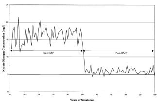
Figure 11–Comparison of pre-BMP and post-BMP annual average nitrate-nitrogen concentrations in leachate at Site E.
