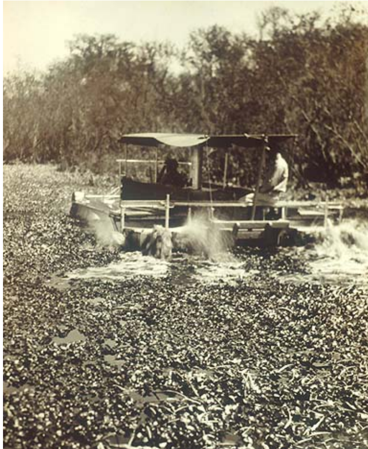
Figure 2 – Water hyacinth shredder in the Withlacoochee River, circa 1940. Photo by United States Army Corps of Engineers, as adapted by the University of Florida Center for Aquatic and Invasive Plants. http://plants.ifas.ufl.edu/guide/mechconold7js.jpg
