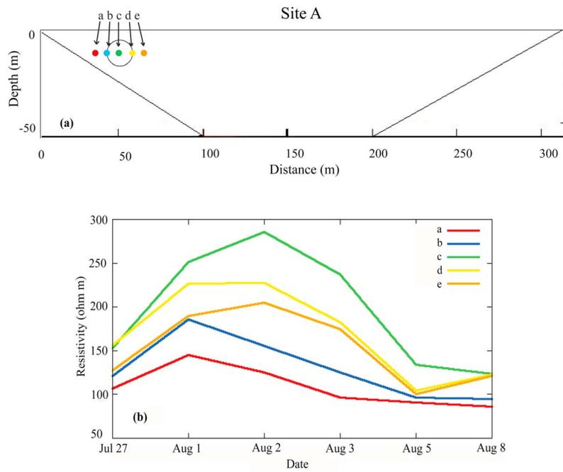
**Figure 4.** Point resistivity (ohm m) measurements through time for Site A. (a) Locations of the points with respect to the subsurface profile and (b) a plot of resistivity data. Point C is in the middle of the projected conduit shown on Figure 3, Point B and D are at  $\pm 10$  meters from Point C, Points A and E are  $\pm 20$  meters from Point C.
