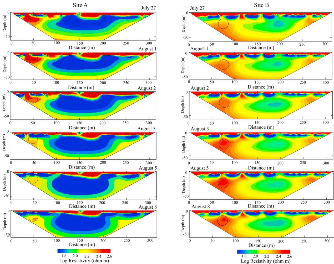
**Figure 3.** Electrical resistivity tomography inversions for Site A and Site B. Spatial distribution of resistance (ohm m) over time between July 27th and August 8th. Estimated karst conduit locations are shown by black circles and are not to scale. Resistivity values (ohm m) are shown in log space.
