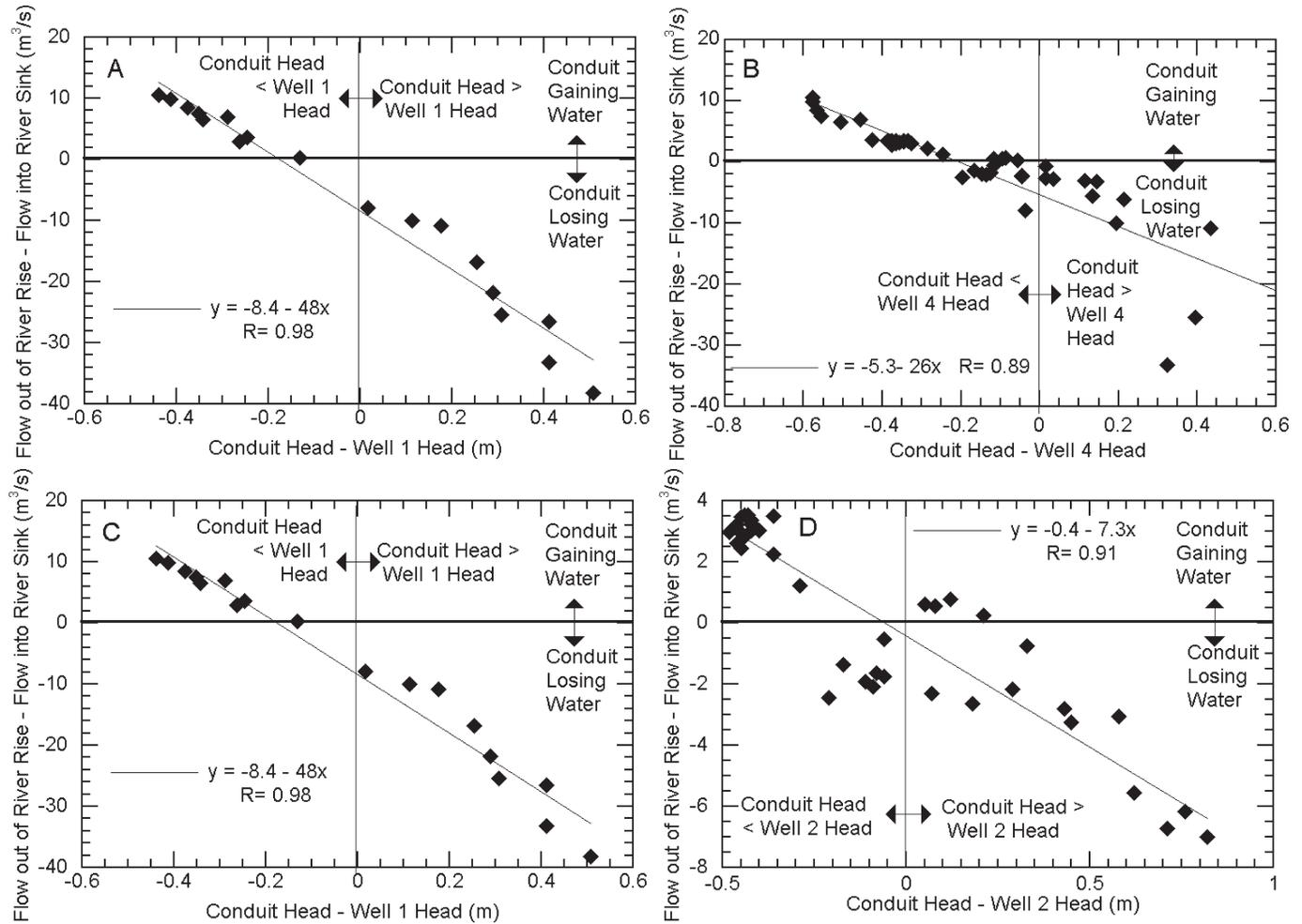
Figure 6. Relationship between change in conduit gains and losses and head differences for (A) Tower Well, (B) well 4, (C) well 1, and (D) well 2.
