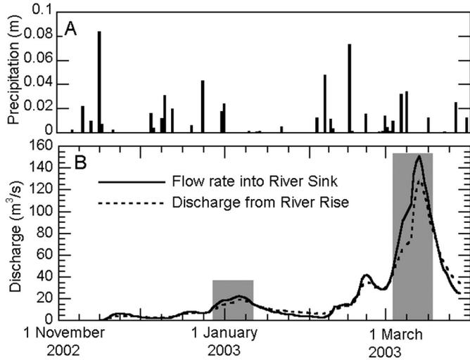
Figure 3. Precipitation and Santa Fe River discharge data for November 2002 to March 2003. (A) Daily precipitation recorded at O'Leno State Park. (B) Inflow rates into Santa Fe River Sink and discharge rates from River Rise. Shaded areas show time intervals when output from the River Rise exceeded input to the River Sink.
