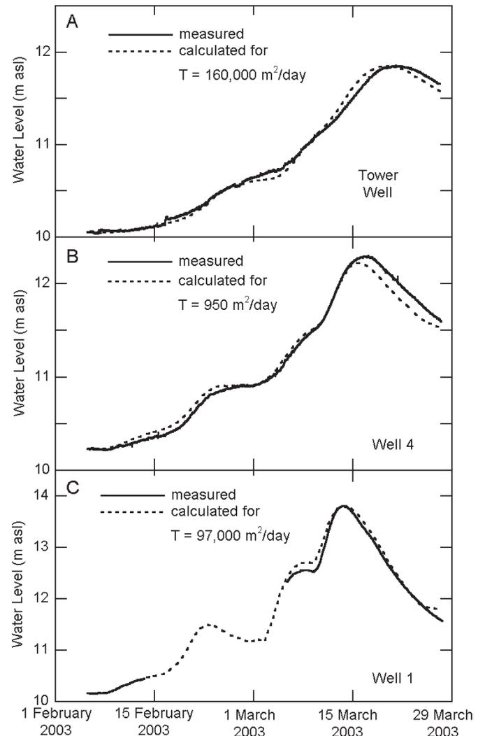
Figure 5. Comparison of measured and calculated water levels for (A) Tower Well, (B) well 4, and (C) well 1. T—transmissivity.
