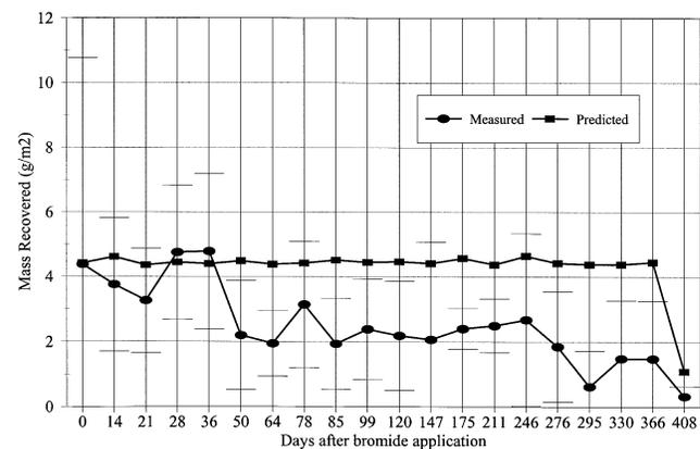
**Figure 2**—Comparison of measured and predicted bromide mass recovery.
