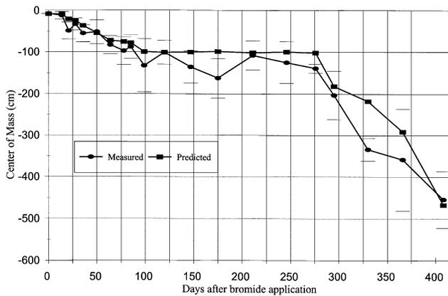
Figure 3—Comparison of measured and predicted movement of the bromide center of mass.
